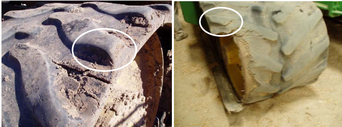
Typical wide track uneven wear
