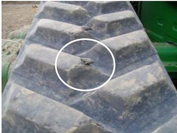
Acute Inner Angle causing inner edge damage
